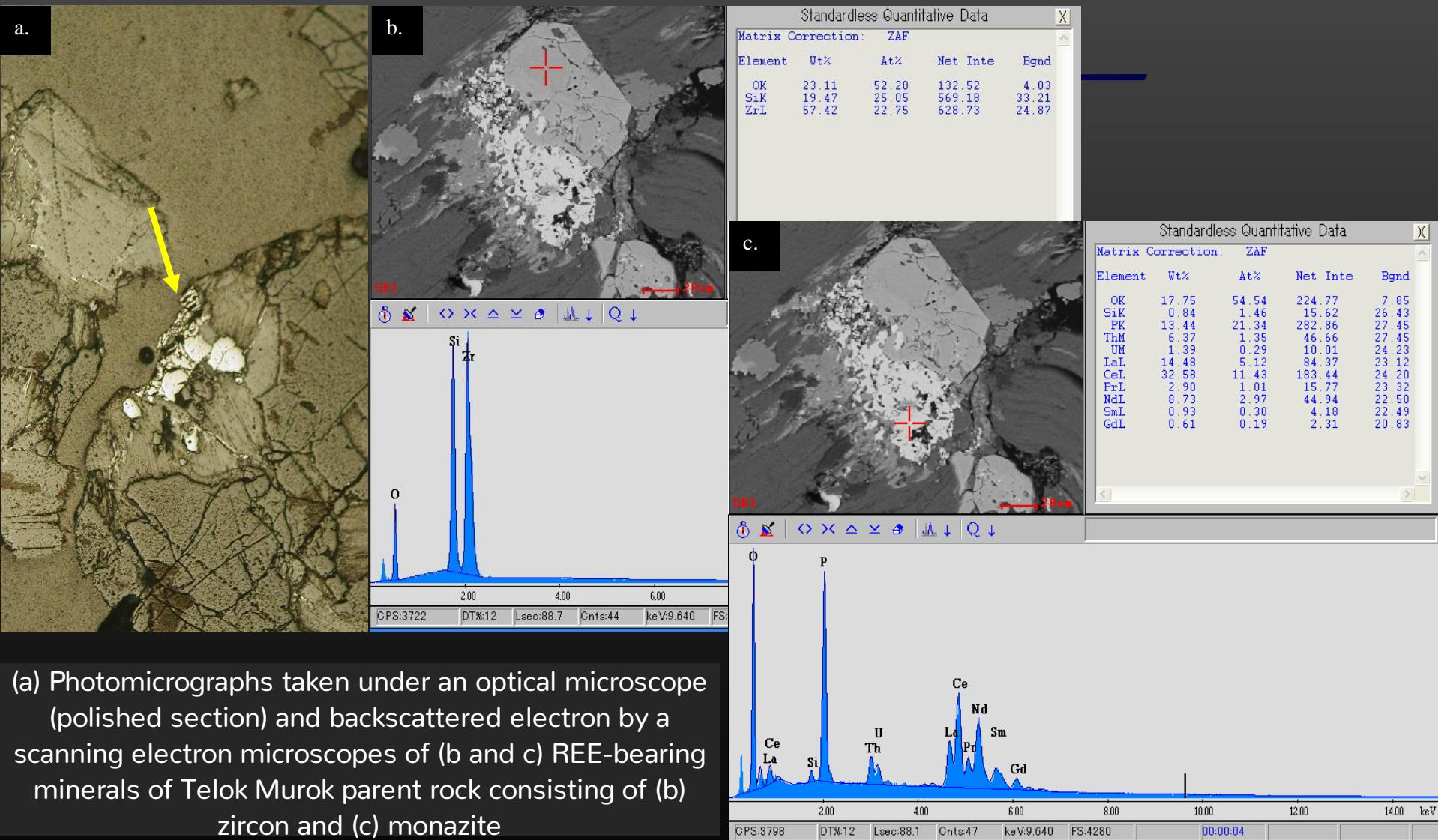
(a) Photomicrographs taken under an optical microscope (polished section) and backscattered electron by a scanning electron microscopes of (b and c) REE-bearing minerals of Telok Murok parent rock consisting of (b) zircon and (c) monazite
