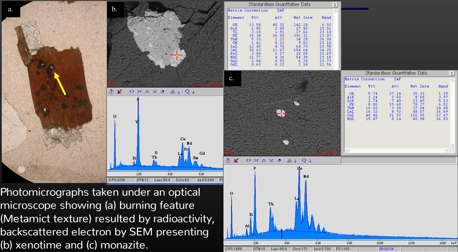
Photomicrographs taken under an optical microscope showing (a) burning feature (Metamict texture) resulted by radioactivity, backscattered electron by SEM presenting (b) xenotime and (c) monazite.
